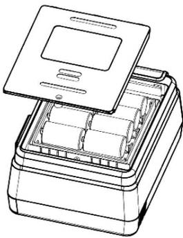
Figure 8. Battery Replacement
