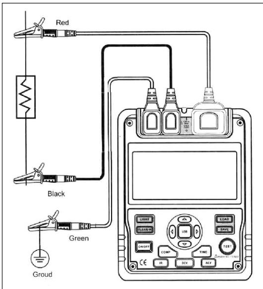
Figure 5. Insulation Resistance Measurement
