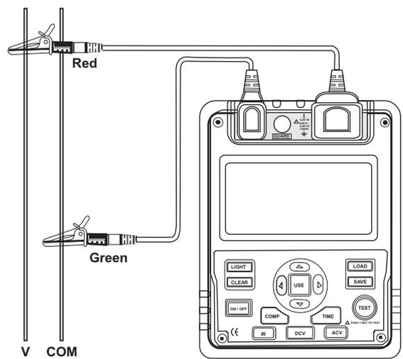
Figure 4. Voltages Measurement
